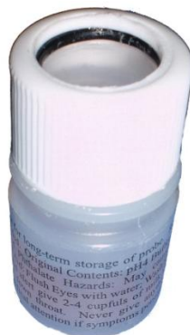
Small bottle filled with pH 4 buffer solution for pH bulb storage
